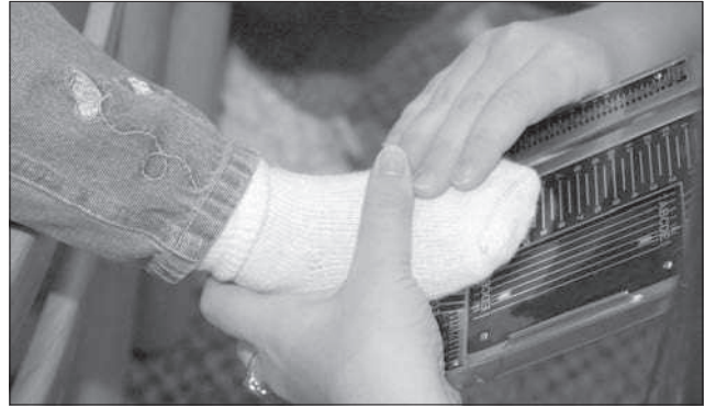
Brannock foot measuring device
